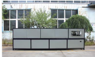
The machine can finish roving guiding, impregnation, preforming, winding, heating, pulling, fix-length cutting and products collection actions automatically. The machine produces fiberglass rebar with different sizes.
